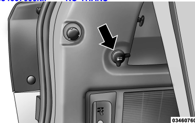
Rear Power Outlet
