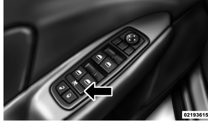
Window Lockout Switch
