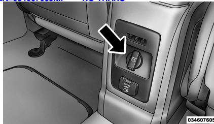
Rear Power Outlet
